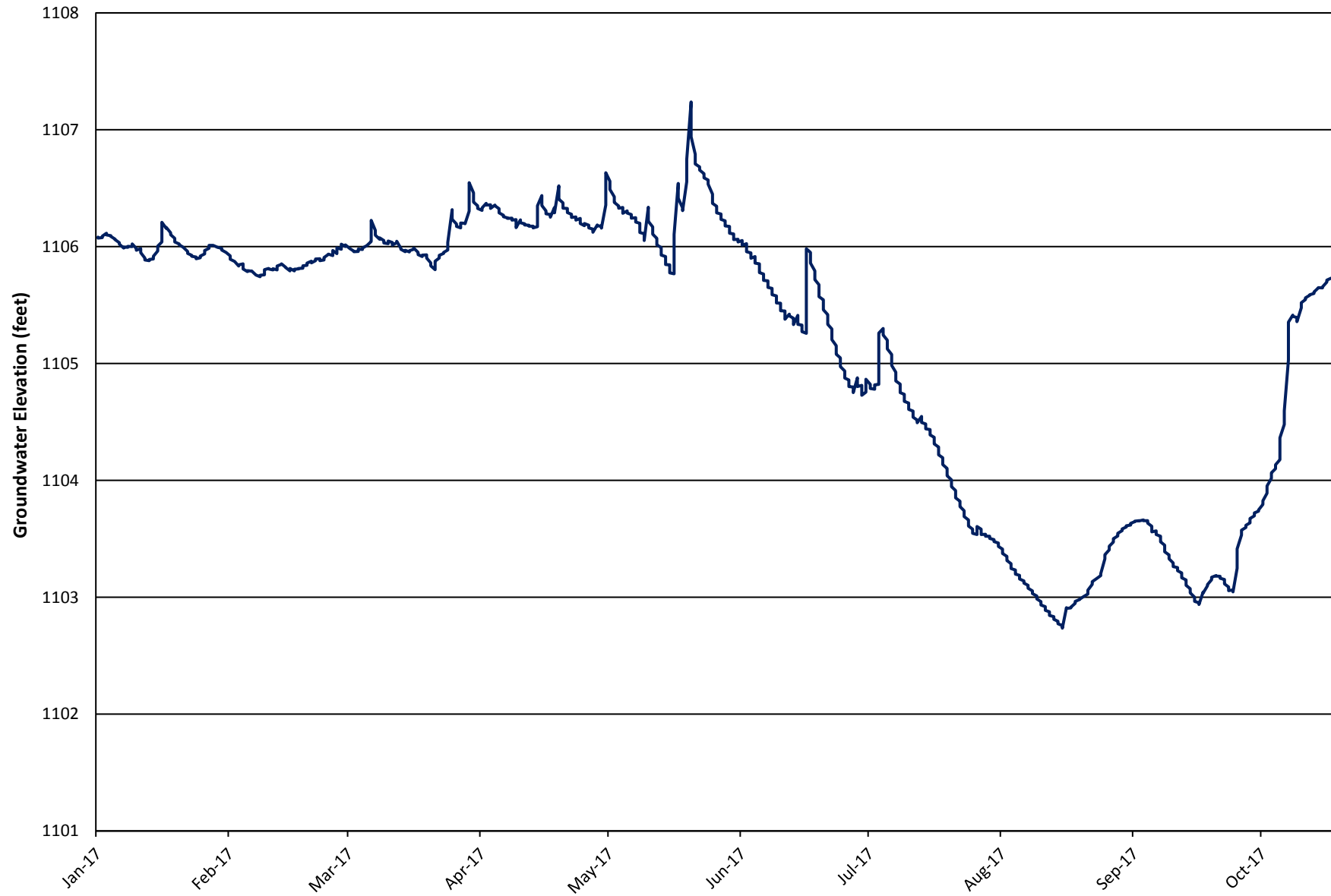
Figure 3 Monitoring Well Readings for MW 90-07 in Douglas County (January 1, 2017 thru October 17, 2017)
