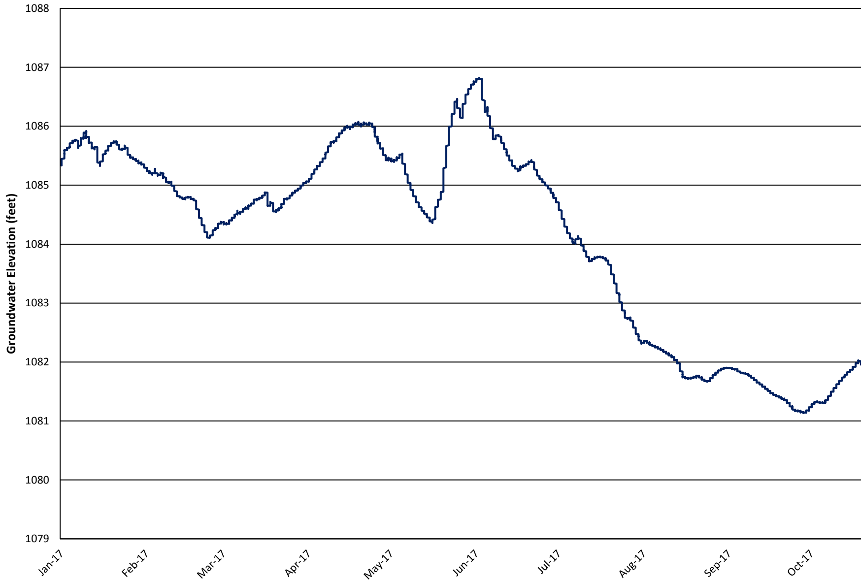
Figure 10 Monitoring Well Readings for MW 94-04 in Saunders County (January 1, 2017 thru October 19, 2017)
