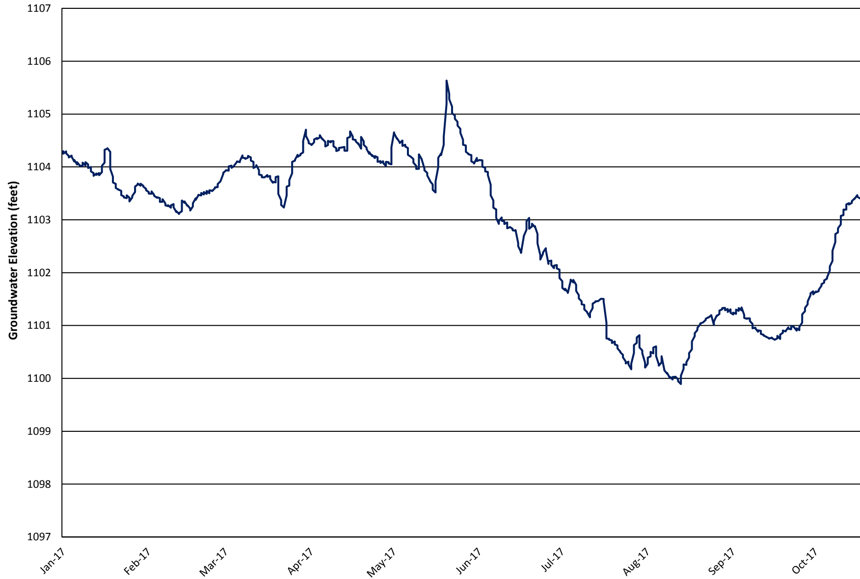
Figure 8 Monitoring Well Readings for MW 94-02 in Douglas County (January 1, 2017 thru October 17, 2017)
