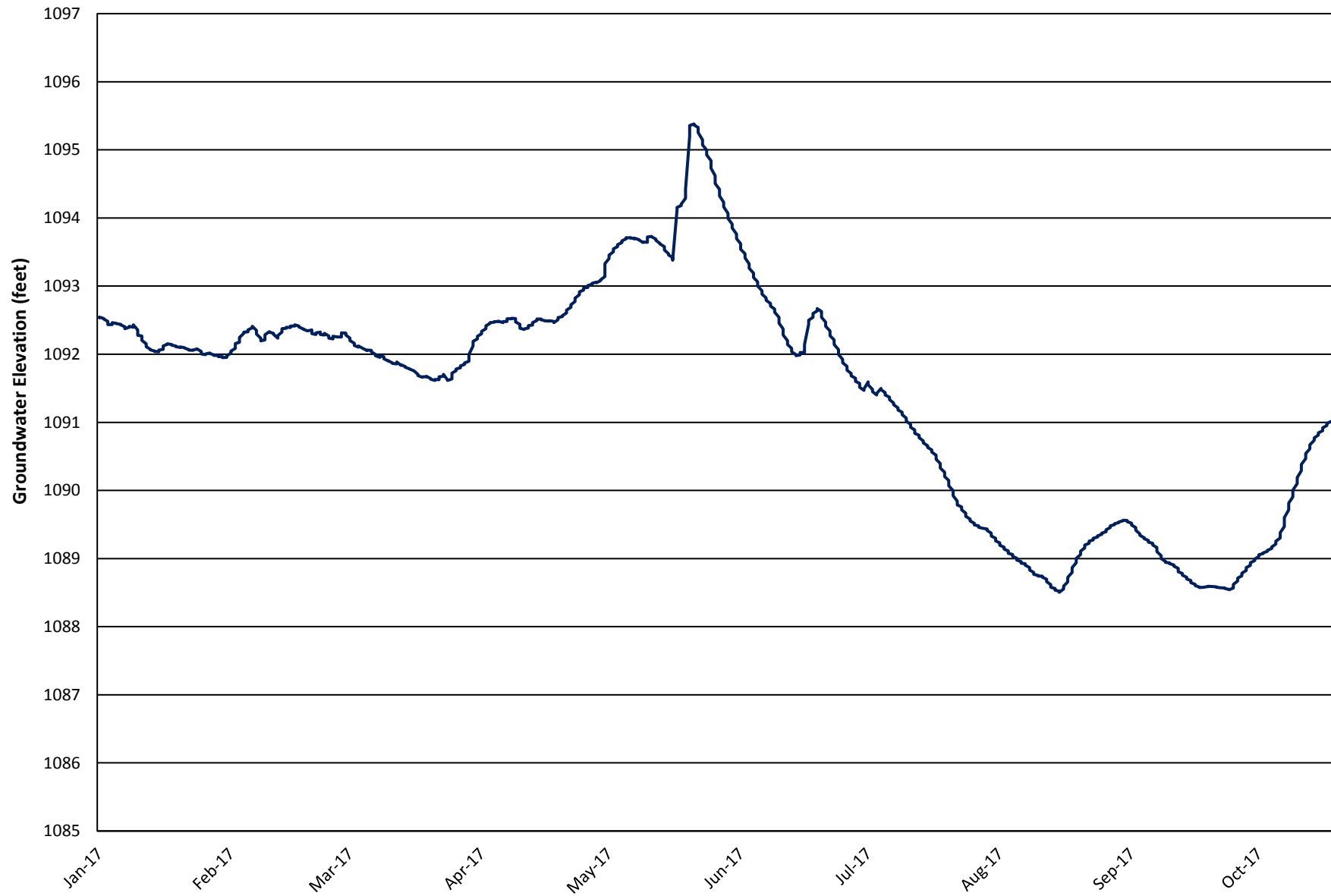
Figure 4 Monitoring Well Readings for MW 90-10 in Saunders County (January 1, 2017 thru October 18, 2017)
