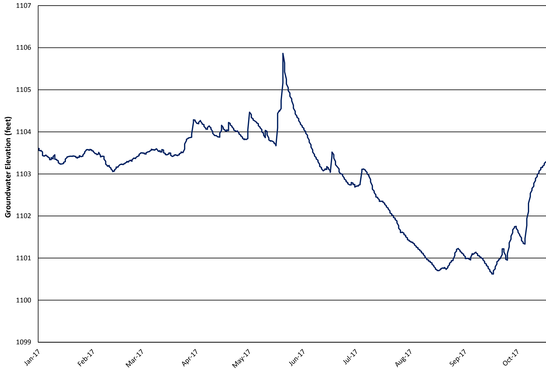
Figure 17 Monitoring Well Readings for MW 05-25 in Douglas County (January 1, 2017 thru October 17, 2017)
