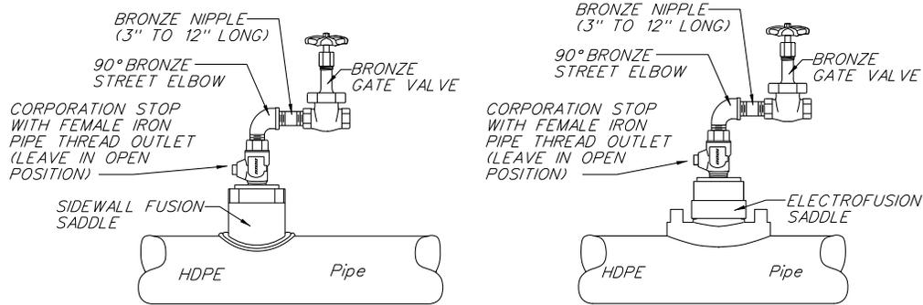
NOTE: Tap shall be made with a manual tapping machine and a shell-type cutting bit designed for HDPE pipe. Hand-held drills shall not be used.
