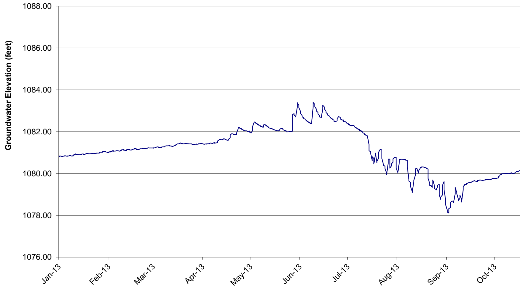
Figure 12 Monitoring Well Readings from MW 94-06 in Saunders County (January 1, 2013 thru October 17, 2013)
