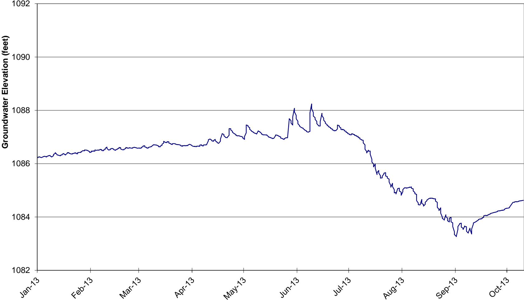
Figure 21 Monitoring Well Readings for MW 06-28 in Douglas County (January 1, 2013 thru October 10, 2013)
