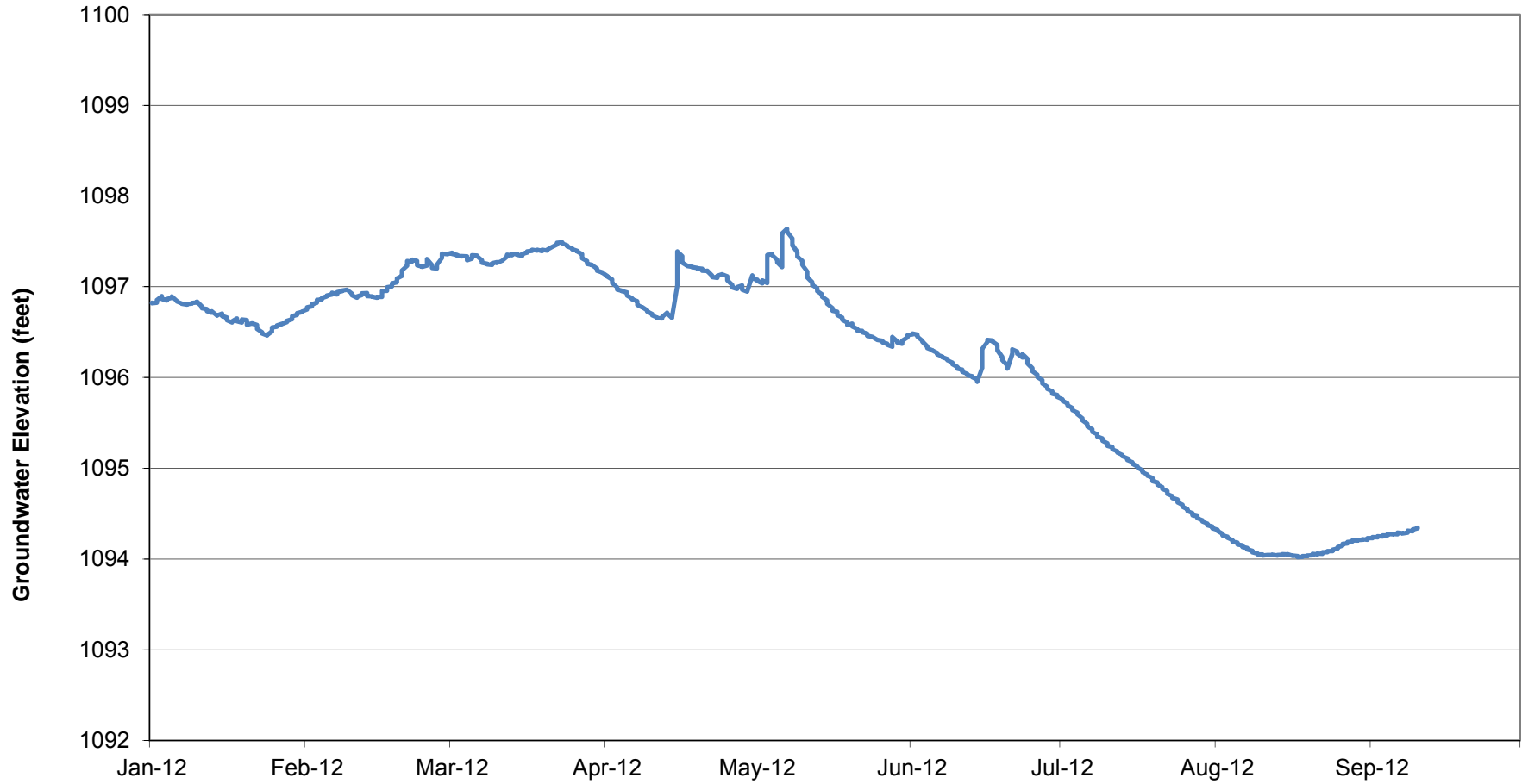
Figure 18 Monitoring Well Readings from MW 05-24 in Douglas County (January 1, 2012 thru September 10, 2012)
